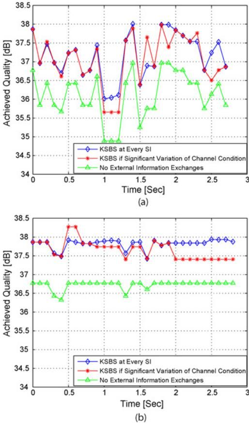
Fig. 3. Achieved quality based on Algorithm 2. (a) Large variation of channel condition. (b) Small variation of channel condition.
