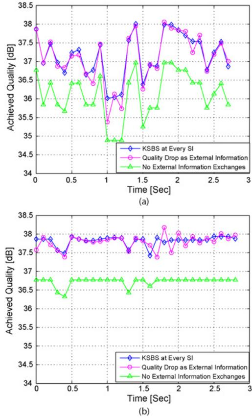
Fig. 4. Achieved quality based on Algorithm 3. (a) Large variation of channel condition. (b) Small variation of channel condition.
