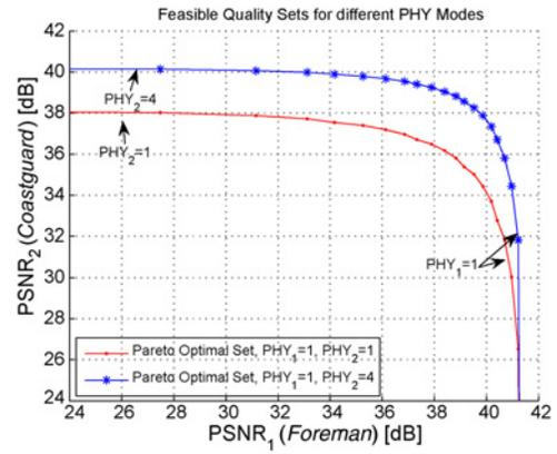
Fig. 1. Achievable feasible quality sets for two WSTAs. WSTAs 1 and 2 transmit *Foreman* and *Coastguard* sequences [common intermediate format (CIF)] under the channel SNRs of 18 dB and 23 dB, respectively.  $\text{PHY}_i$  denotes the PHY mode choice of WSTA  $i$ . The duration of SI is 100 ms (i.e.,  $t_{SI} = 100$  ms) in this example.
